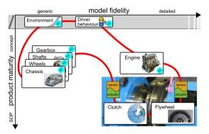
Validation approach to combine different product maturities and accuracies of the subsystems using the Power Pack Test Bench
