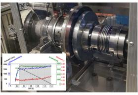
Measurement of the temperature distribution using fiber optic sensing technology with high spatial measurement density
